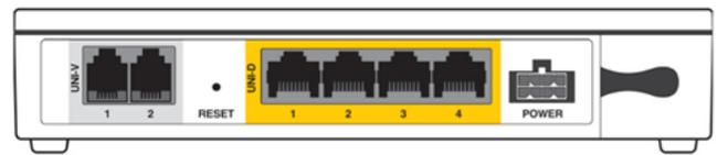
Using an ethernet network cable connect your router from its WAN port to the relevant Uni-D port on the NBN Connection Box. We generally activate the next available Uni-D port – starting with Uni-D 1. We will detail your Uni-D port number in our emails to you.
