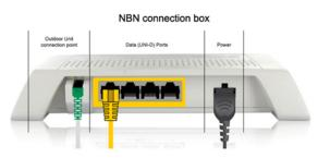
Using an ethernet network cable connect your router from its WAN port to the relevant Uni-D port on the NBN Connection Box. We generally activate the next available Uni-D port – starting with Uni-D 1. We will detail your Uni-D port number in our emails to you.
